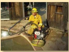
backwards out of the hose. This is very helpful in initially establishing flow through the pump and maintaining flow if you need to stop and start the pump. The discharge should be compatible with your fire department's fittings.
